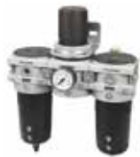
Filter + Regulator + Lubricator Combinations 40 micron element, 12 bar Regulator + Gauge and Wall Mounting Bracket
